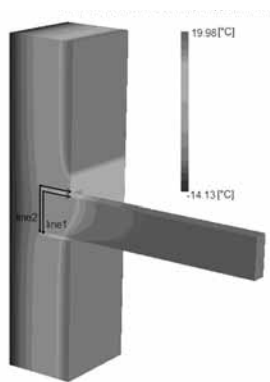
Fig. 3. Simulation of temperature distribution in stationary condition – horizontal section
