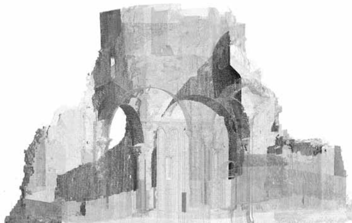
Fig. 4 Image of the points cloud obtained by the three-dimensional survey made with 3D laser scanner, in 2011.
