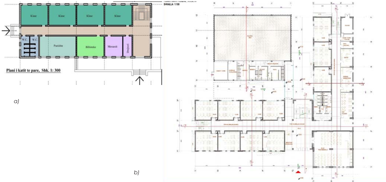
Figure 10: a) Above: Scheme of Type '61, asymmetrical primary school, the year 1961, arch, Valentina Pistoli, b) Below: School Ahmet Gashi, 2012, Ground floor plan.
