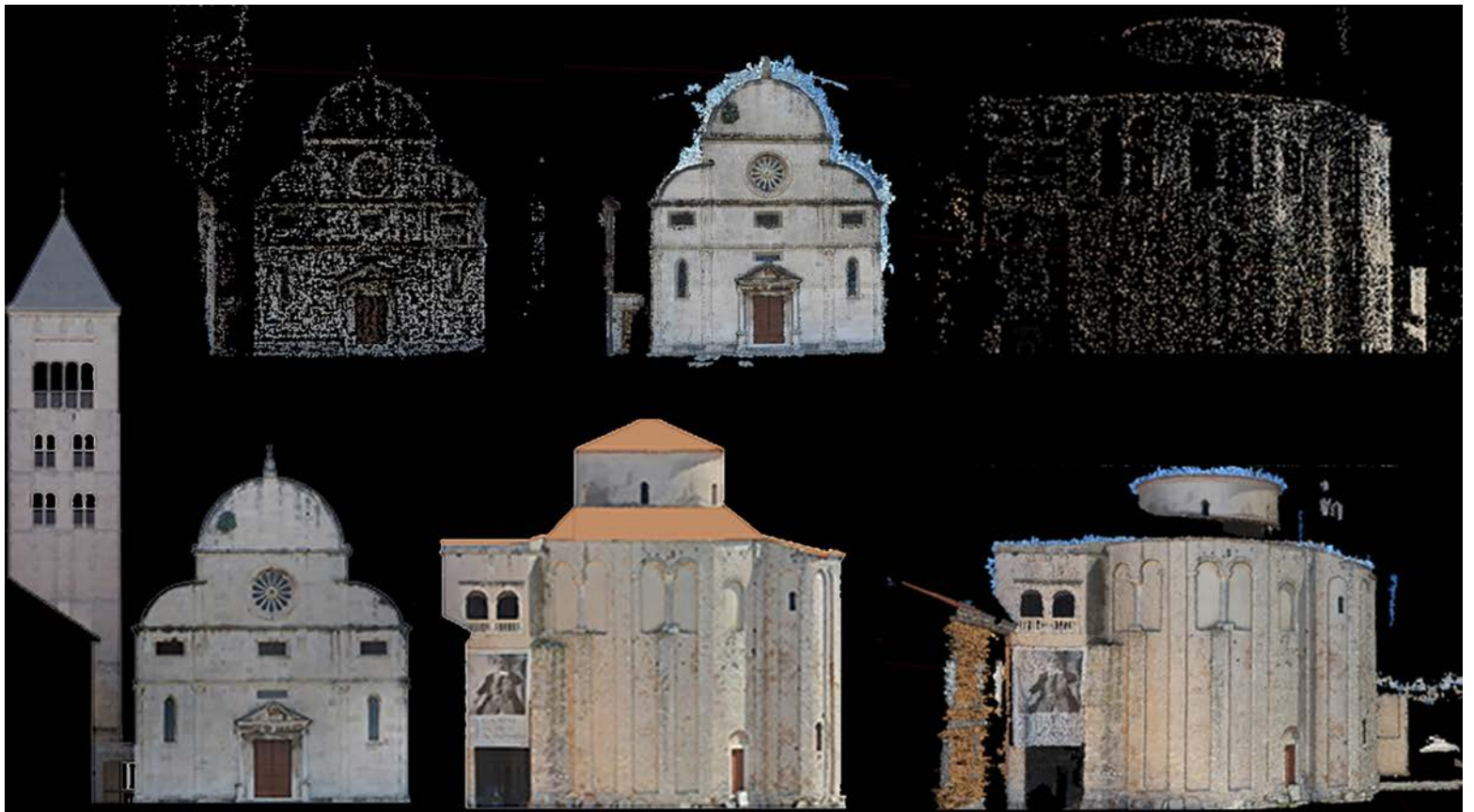
Figure 5. Processing of point clouds and orthomosaics from photogrammetric survey.
