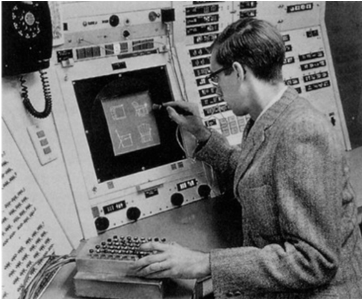
Figure 6. The first CAD system, Sketchpad by Ivan Sutherland, 1963, developed at the Massachusetts Institute of Technology.
