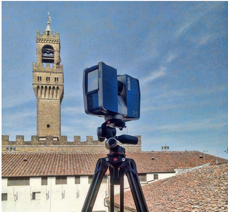
Figure 1. A Laser Scanner unit (Cam/2 Faro X330 Phase Shift measuring technology with an operative range up to a distance of 330 metres) during the survey of Palazzo Vecchio in Florence, August 2019. Source: G. Verdiani.
