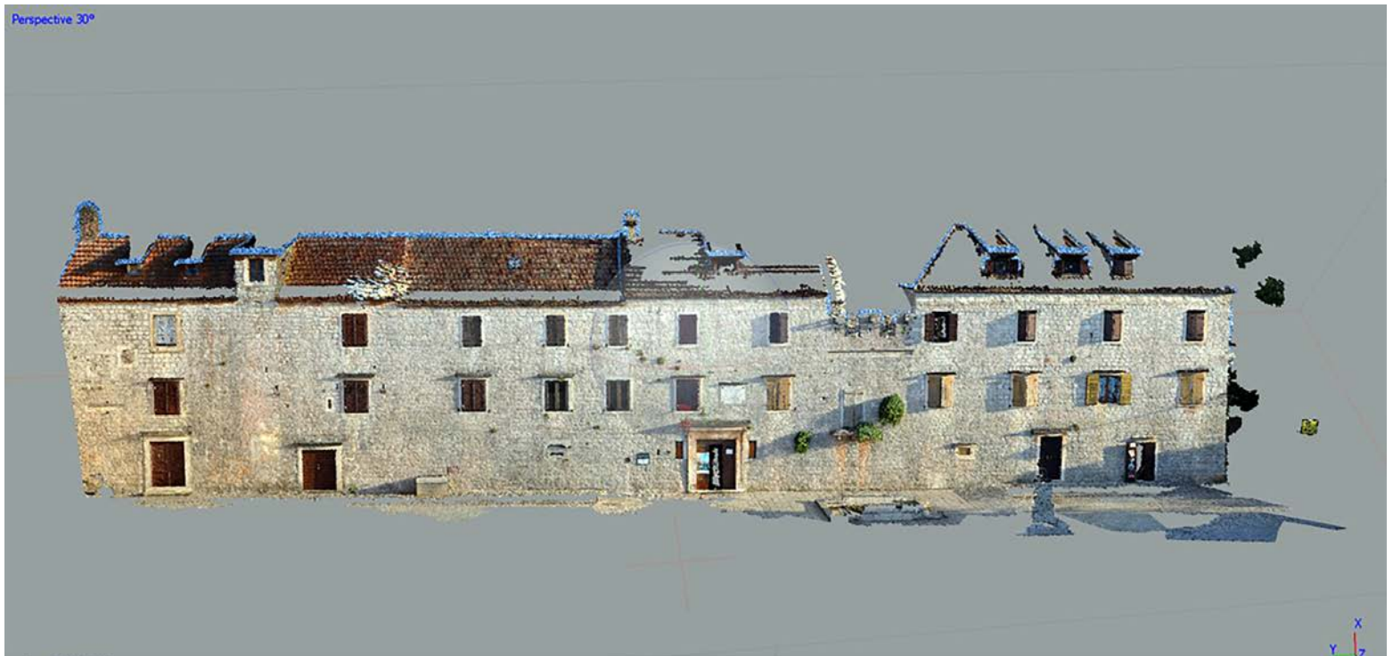
Figure 1. Point of cloud made with photogrammetric representation software. Main prospect of the Tvrdalj Fortress in Hvar.
