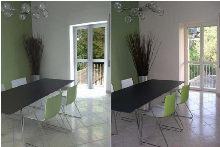
Figure 7. Same 3D digital model, rendering in Biased (on the left) and Unbiased (on the right) graphic engines.
