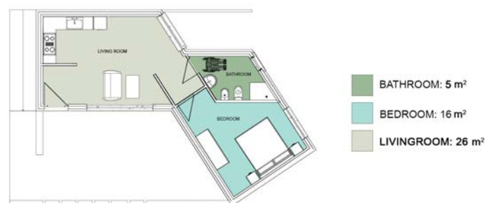
Figure 1. Solar House - Ground floor functional layout
