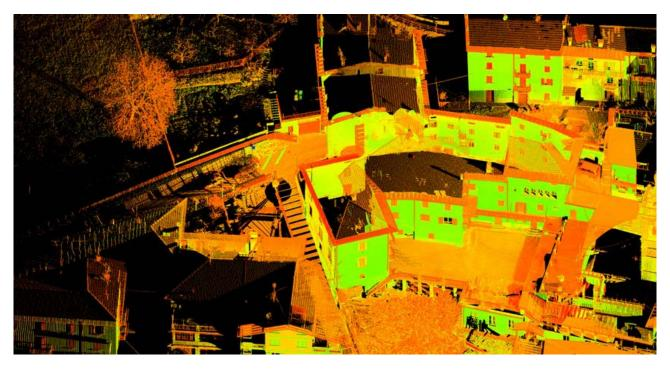
Fig. 2: Scan performed by terrestrial laser scanner and displayed in the form of points of cloud.
