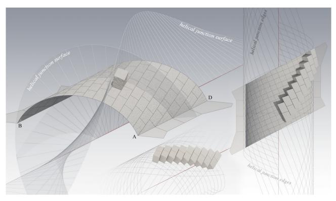
Fig. 4: The helical's serial texture is achieved through a rototranslatory movement of an ashlar type.
