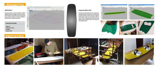
Fig. 4: Design and pictures showing work in progress and final prototype of a kitesurf board realized in Dibond (Students: R. Nocolò, A. Prigiobbo).
