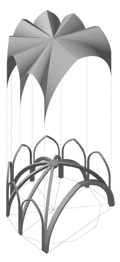
Fig 5. Volume reconstruction of the apse.
