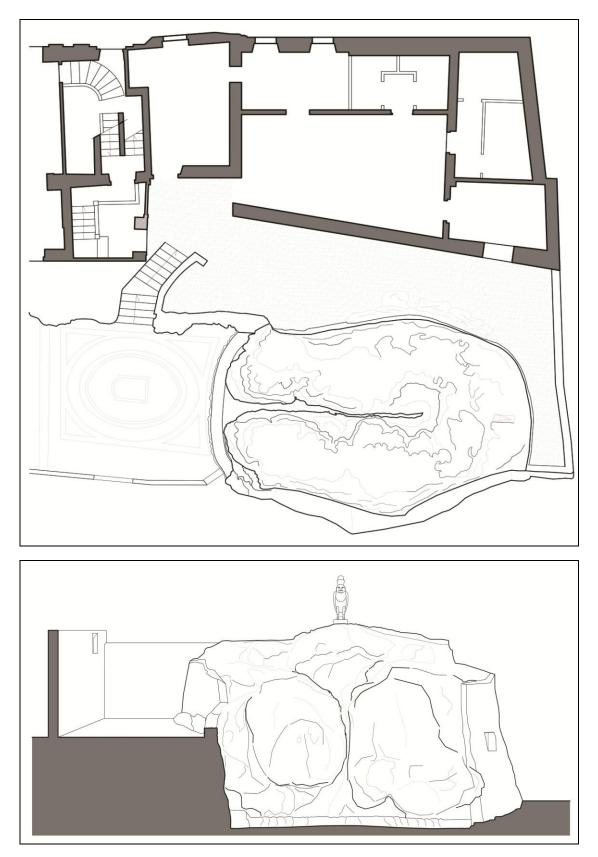
Fig: 6, 7: Plan and elevation derived from laser scanner simplified calculations for the scale of representation.
