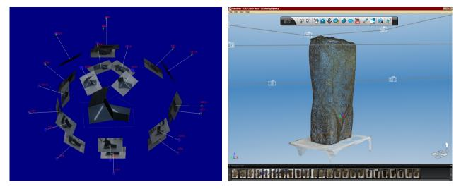
Fig. 1, 2: Position of the photographs on textured 3d model built with *PhotoModeler Scanner* of EOS System; and view of the mesh calculated by *123d* of Autodesk and position of some photographs. In both, we see how the pictures surround the sculpture in two parallel rings separated in height each other the corresponding base for the relationship base/distance of 0,15.
