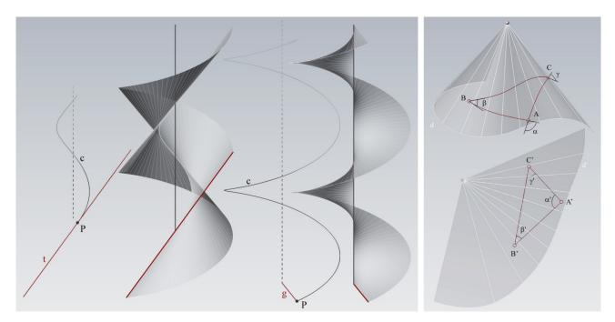
Fig. 1: From left to right; developable helical and ruled helical, genesis in comparison and properties of developable applied to the case of a generic cone.
