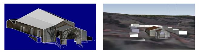
Fig. 8: Santa Susanna, phases of modeling: photo modeling and georeferencing of the model
