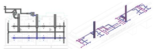
Fig. 7: Detail of the Revit's MEP model, concerning a piece of the HVAC system of the Cittadella Politecnica
