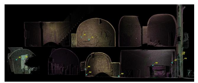
Fig. 11: Carbonara. Building in Corso Vittorio Emanuele: longitudinal section from laser scanning
