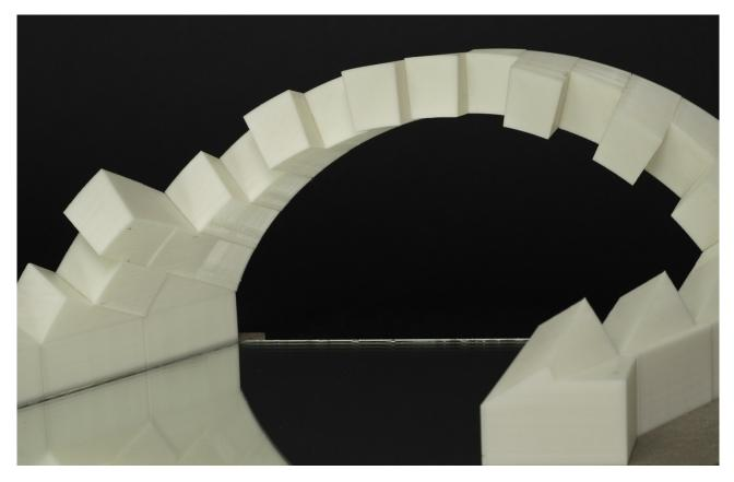
Fig. 7: Print stereolithography 3D of the helical apparatus.
