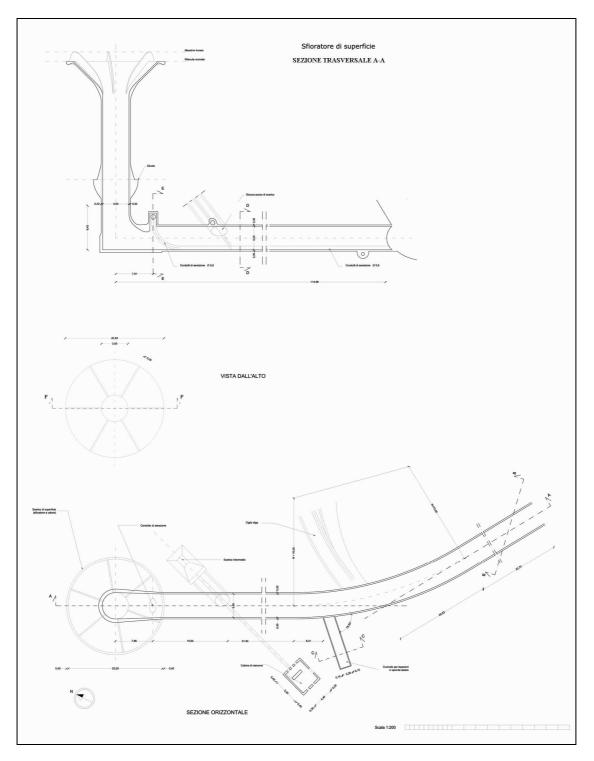
Fig. 7: Surface overflow: view from above and sections
