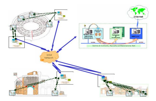
Fig. 2 shows the general configuration of the monitoring system with the Data Acquisition Position connection.
