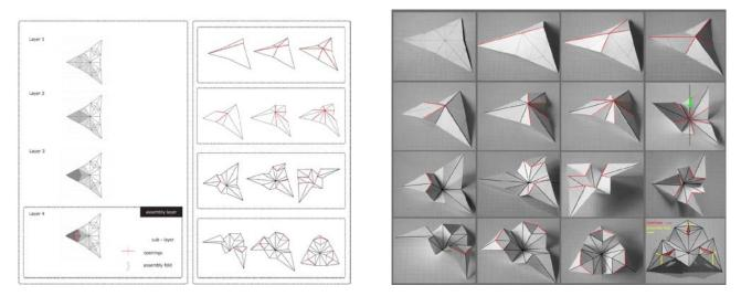
Fig. 3: Fold layer strategy, fold sequence strategy and component's transformation from a flat to a folded state.
