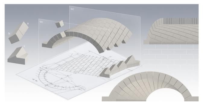
Fig. 5: Construction of the three types of ashlars that make up the apparatus.
