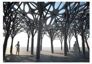
Fig. 1: Quad Meshes in Architecture by Benjamin Schneider (TU-Wien) created using Generative Components. [3] Fig 2: Part of the project "Blurring Structures" by Prof. Grohmann (University of Kassel, Faculty of Architecture, Departement of structural design). The generating script is based on Aristid Lindenmeyer's L-System. In order to dimension the structure automatically, a RhinoScript-RSTAB-Interface was developed. [4]
