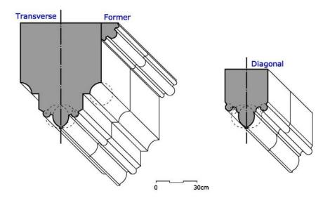
Fig. 4: Moulding of the ribs
