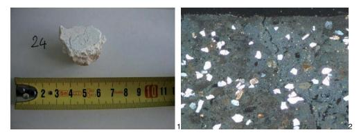
Figure 5. (1) Image of the sample 24: Ottoman finishing plaster; (2) thin section image of the same, 40x. The sample is in a state of sufficient preservation .
