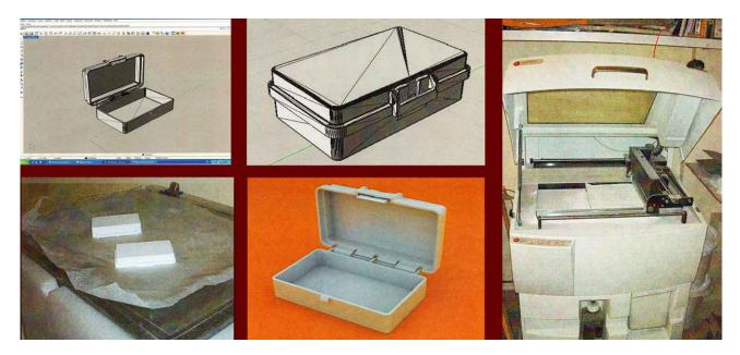
Fig. 5: Renders and prototyping of a 24 hours suitcase in reduced scale (Stereolithography) (Student: G. D'Amico)
