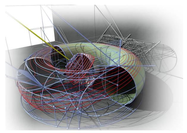
Fig. 11: Construction of the torus' isophotes
