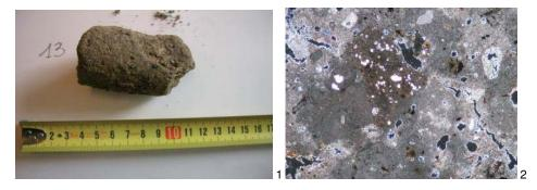
Figure 4. (1) Image of the sample 13 as it is: Crusader bedding plaster ; (2) thin section image of the same, 40x. The sample is in good condition.
