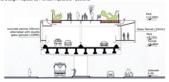
Fig. 12: Generic Section of the project, showing the tunnel with a gallery on one side. Source: Frentes Arquitetura.
