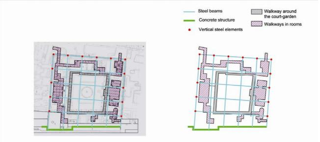
Fig. 3: Périgueux, *domus* de Vésone, diagrams of the structure and the paths inside the new protective structure.
