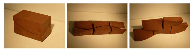
Fig. 7: Single components of unfired (green) terracotta and assembly simulation of a doubly-curved wall section.
