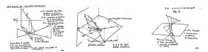
Figg. 11, 12, 13: Drawings by Xenakis, describing the geometrical analysis of the hyperbolic paraboloids.
