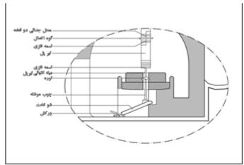
Figure 5.Detail of turbine of windmill. Writer)
