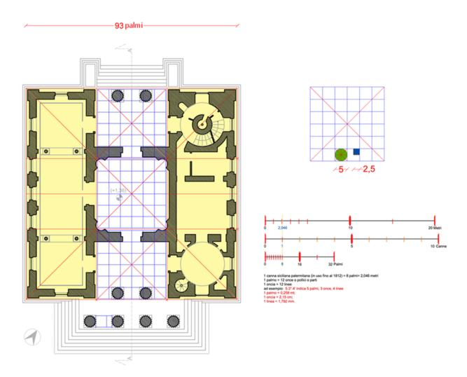
Fig. 3: On the left, the floor plan of representation in the *Gymnasium*. Top right, graphic design of the modular system that regulates the division of space, below, scales, and comparing unit conversion.
