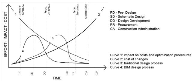
Fig. 1: Macleamy curve comparing the course of the current design process with the results of using a BIM approach in terms of effort, timescales and costs
