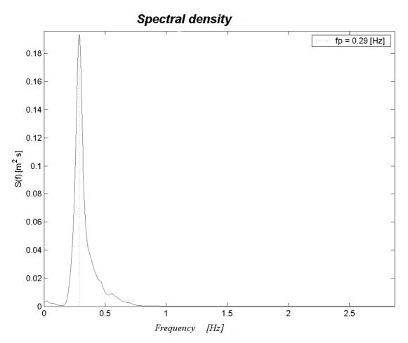
Fig.1 Wave off frequency spectrum.
