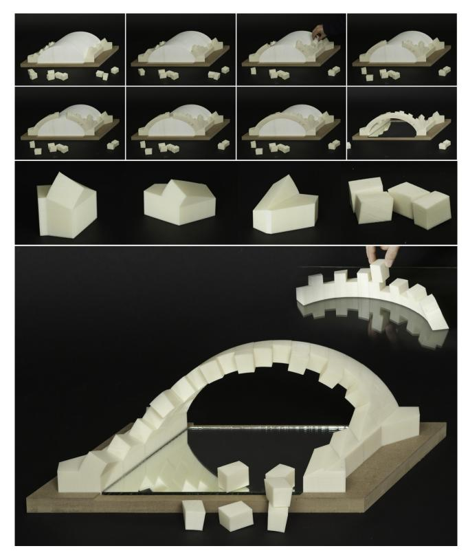
Fig. 6: Print stereolithographic 3D of the helical apparatus and relative phases of assembly.
