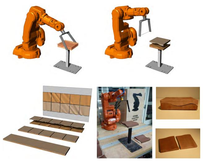
Fig. 9: Design speculations and robotic fabrication of complex terracotta tiles.
