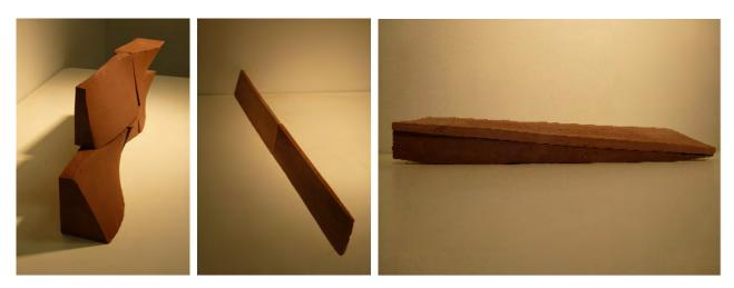
Fig. 10: Prototypes of a doubly-curved wall section and curved louvers made of wire-cut green terracotta.
