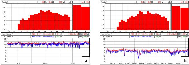
Fig. 4: a) Time history and 1/3 octave band spectrum of the binaural audio recordings carried out a) in a position very close to the Giglio; b) in a position in which the obelisk could not be seen.
