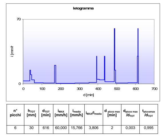
Figure 4 – Pluviogramma, ietogramma and shower parameters: 12.11.2006
