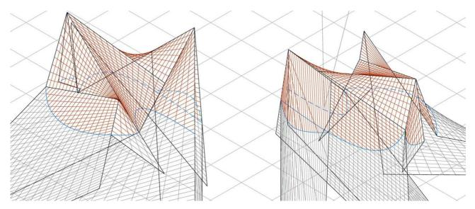
Figg. 23, 24: Wireframe models of the Pavilion with the integral extension of the hyperbolic paraboloids under the groung level (elab. M. and M.S. Soraperra).
