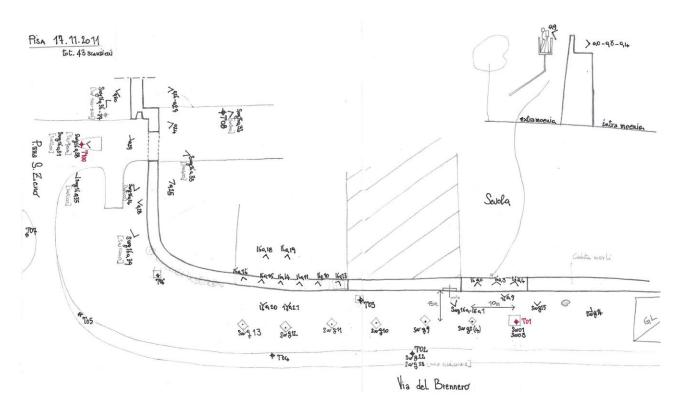
Fig. 2: Points of view or scan worlds of 3D laser scanner, GPS, and spatial station in a survey sketch (A. Avella, 2011).
