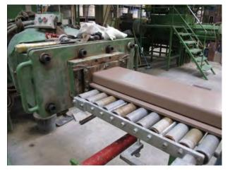
Fig. 1,2: Industrial processes of clay extrusion and cutting.
