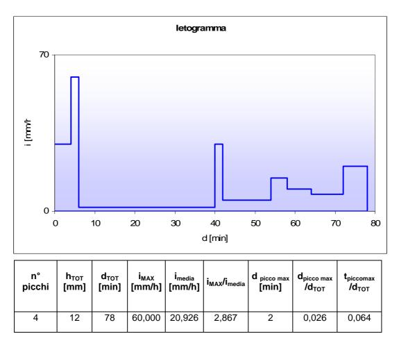
Figure 3 – Pluviogramma, ietogramma and shower parameters: 17.09.2006
