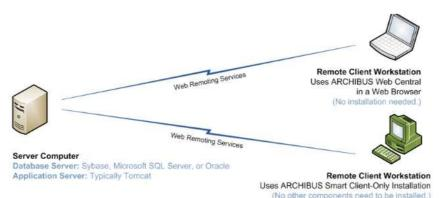
Fig. 4: Client-Server structure of Archibus FM application
