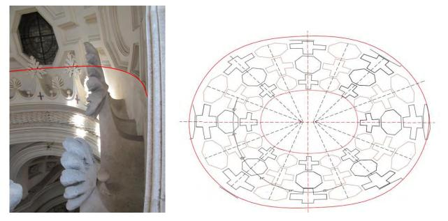
Fig. 5: Drum cornice and impost oval (red) (C. Falcolini)Fig. 6: Plan drawing where coffers alignments are highlighted following 5 centres
