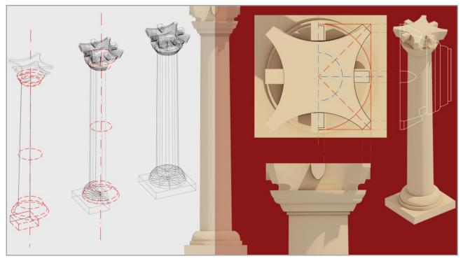
Fig. 9: Three-dimensional modeling of a Nabataean column.
