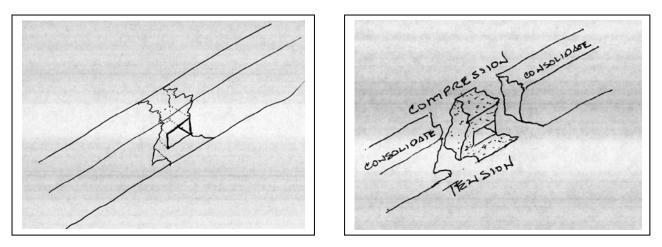
Fig. 12,13: Beam with completely deteriorated area at a mortise; Exploded view with a loose casting to fill the missing portion – if tightly assembled, in theory it only needs a tension connection at the bottom to function. See Fig. 14-17.
