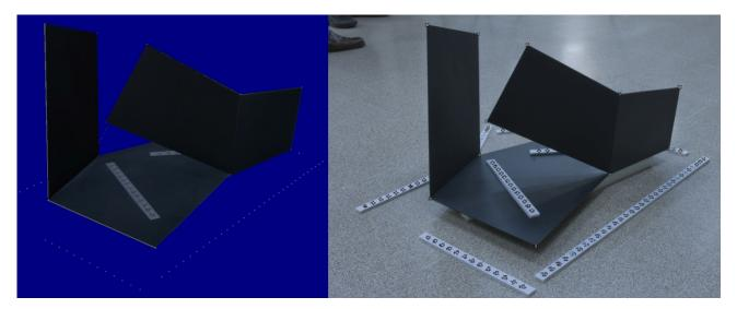
Fig. 4: Model constructed manually by assigning control points in all photographs. These are both coded targets that were placed to facilitate the orientation of the cameras, as the vertices that define the geometry of the sculpture.
