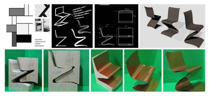
Fig. 2: The *Tape Chair 2010* Design is conceived in carbon fibre, along the lines of the *Zig - Zag* revisitation to which it adds the *Panton Chair* shapeliness, but the prototype, in reduced scale, has been realized in copper foil.
