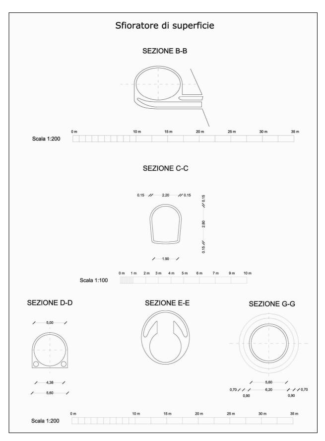
Fig. 5: Surface overflow: cross sections
