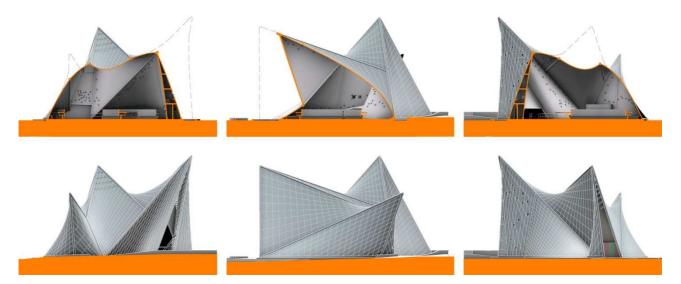
Figg. 25, 26, 27, 28, 29, 30: Vertical sections of the digital model (top) and elevations (bottom) (elab. M. and M.S. Soraperra).
