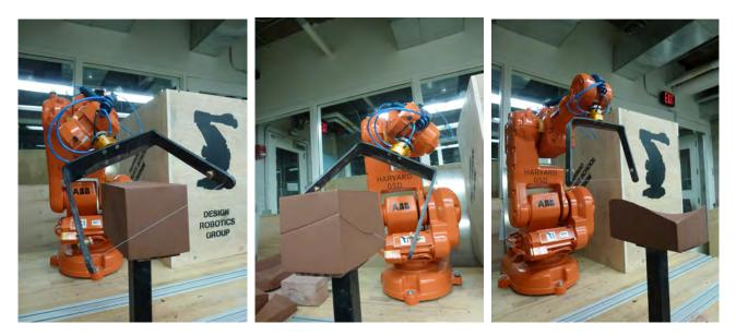
Fig. 6: Robotic fabrication of ruled-surface ceramic units for doubly-curved wall systems.
