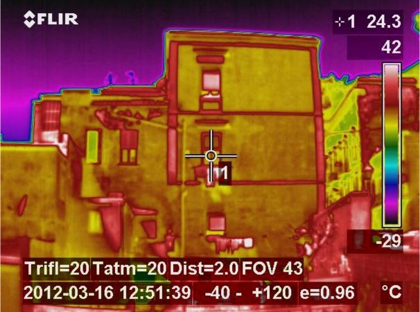
Fig. 9: Sarno (SA), sample block, inner southern front. The thermography IRT proves the masonry stratigraphy.
