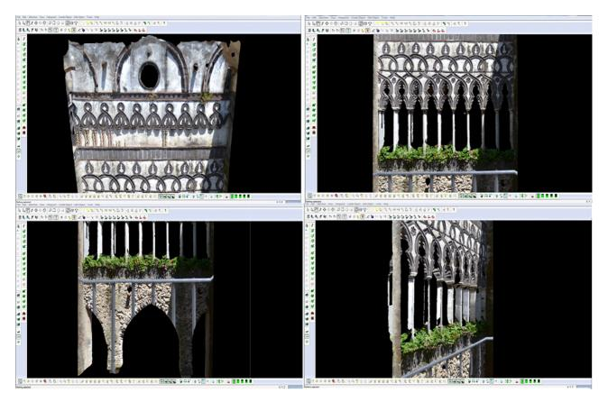
Fig. 6: Views of the photograpic image applied to the cloud of points - mesh
