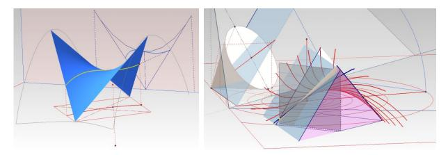
Fig. 9: Hyperbolic paraboloid...
