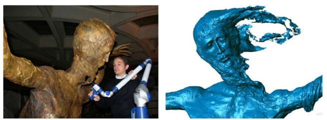
Fig. 35-36: 3D laser scanning action and mesh 3D model by point cloud model (P. Argenziano, Benecon 2011).
