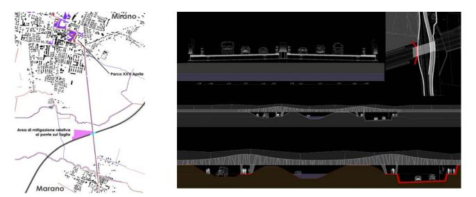
Pic 4 Left: positioning of the bridge in respect of the built-up area. The purple color shows an area which will become a park and is connected to a green area in the centre of Mirano through the passage under the new bridge. Right: section, planimetry and prospects.
