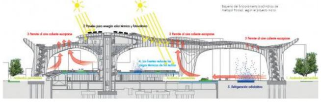
Fig. 12: Function diagram Metropol Parasol bioclimatic, initial project. [26]
