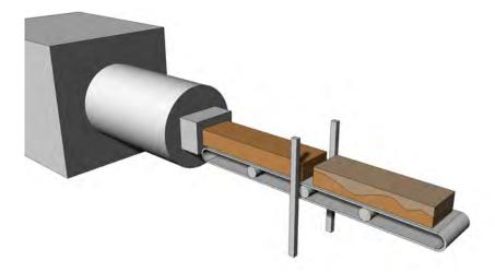
Fig. 3: Envisioned industrial method of automated wire-cutting.
