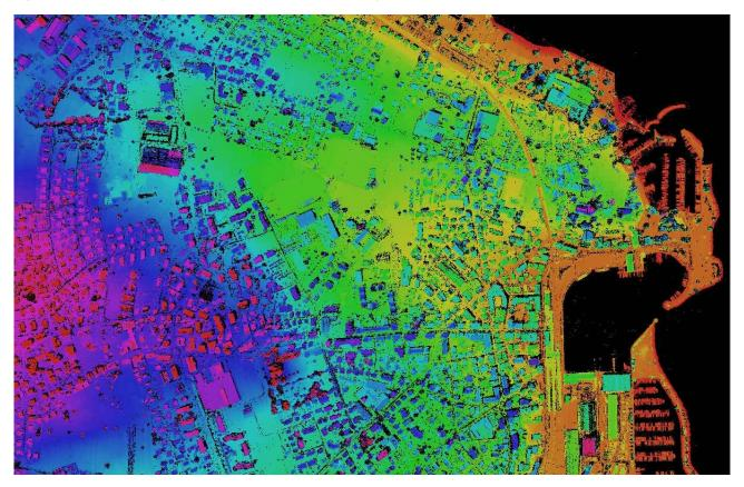
Fig. 3: Scan performed by airborne laser scanner and displayed in the form of points of cloud.
