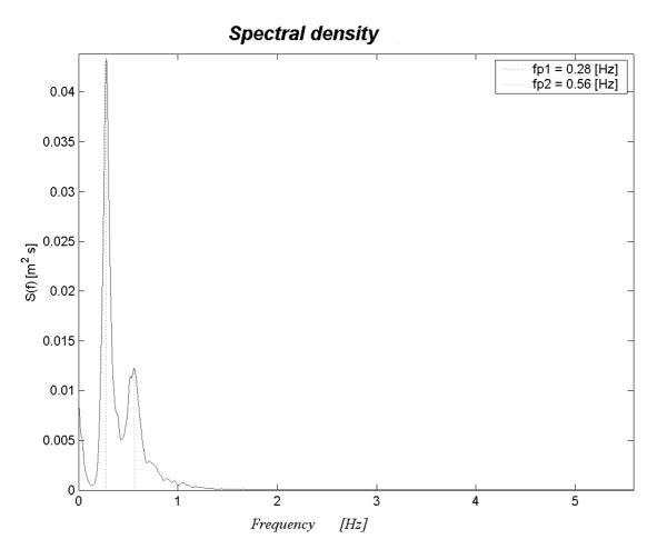
Fig.2: frequency spectrum of the wave after the barrier impact.
