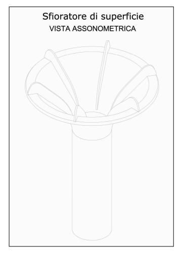
Fig. 6: Surface overflow: orthogonal axonometry
