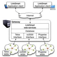
Fig. 3 Software infrastructure scheme to handle heterogeneous Wireless Sensor Networks.
