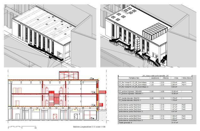
Fig.4. The variable time can be effectively managed within the BIM, as demonstrated by the following documents that compare the status of fact, the future project, demolition and construction section view and extract theme of schedule. (Authors of the virtual model of new classroom design: eng. G. Cangialosi and eng. M. Lo Turco).
