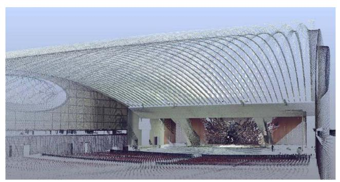
Fig. 28: The 'Aula Paolo IV' point cloud model, perspective projection (P. Argenziano, Benecon 2011).
