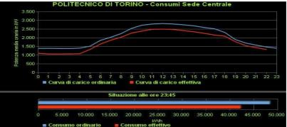
Fig. 1: Representation of the ordinary and effectives consumption on February 17th, 2012, for the Main Campus of Politecnico di Torino [taken from web site: http://smartgreenbuilding.polito.it/]
