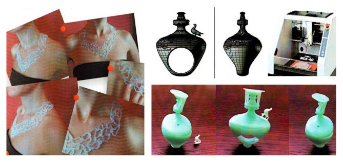
Figg. 9, 10: On the left, a collier realized by the straining of silicon rubbers in ad hoc made mould (Student: B. Frettoloso). On the right, renders and wax models of rings inspired to campanian etrurian archeology, realized by the laser stereolithography (Student: L. Gambero).
