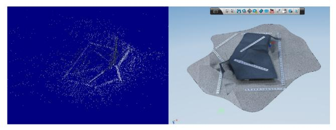
Fig. 3: These images show how the flat black color is a serious problem for the algorithms of calculation of any software, by not recognizing the corresponding homologous points. The images refer to *PhotoModeler Scanner* and *123d* of Autodesk, but have also been tested and *ARC 3D Webservice* and *My3dscanner*. The laser scanner is not able to resolve a point cloud right in these cases.
