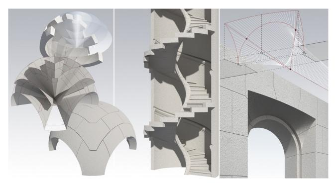
Fig.2: Developable and ruled applied to the case of spherical vaults, the spiral staircases, splayed vaults.
