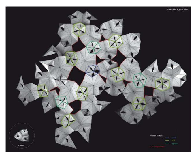
Fig. 5: Assembly A<sub>2</sub> demonstrating a surface element out of three iterative component's rotations.
