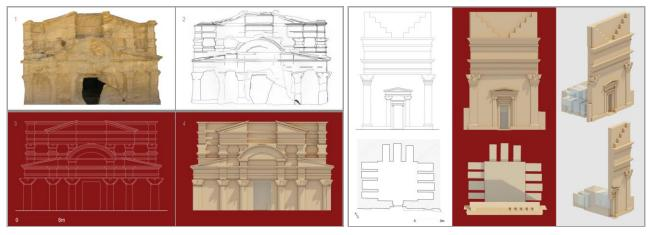
Fig. 10, 11: Bab el Siq Triclinium – Uneishu tomb: photogrammetric survey, geometric survey and rendering images.
