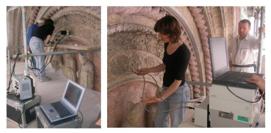
Fig. 1: experimental set-up for in situ measurements at the Palazzo dei Priori by XRF (a) and mid-FTIR (b)
