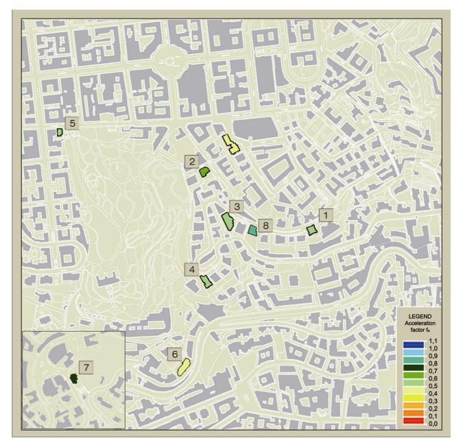
Figure 2. Map showing buildings with colours of their acceleration factor  $f_{a}% =1,1,2,\ldots,n$
