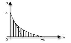
Fig. 5: Stress in the material versus the distance between the faces after the opening.
