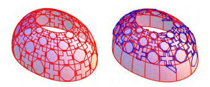
Fig. 9: Three-dimensional model: the shape of the surface is an ellipsoid constructed on the base curve. The average distance of such a model surface from the measured points is around 5 cm.
