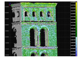
94,271 points of the 98,733 were compared at a range of  $\pm$ 20mm, for 95.48% of the points within the comparison range. The average was 0.170 mm with a standard deviation of 18.09 mm, while all the points converge within 4 times the Std.Dev.
