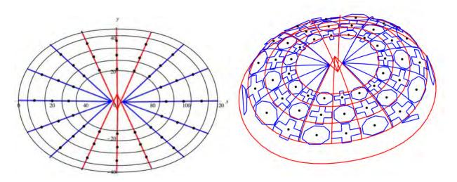
Fig. 10: Plane projection of the baricentral points of crosses and octagons in the new survey for the last three levels. In each sector, these points are almost aligned and have different mutual distance; the lines meet at different points if continued by the same proportion (5/6) for the blue lines and its square (25/36) for the red lines. Red and blue lines have, respectively, the same angular distance.
