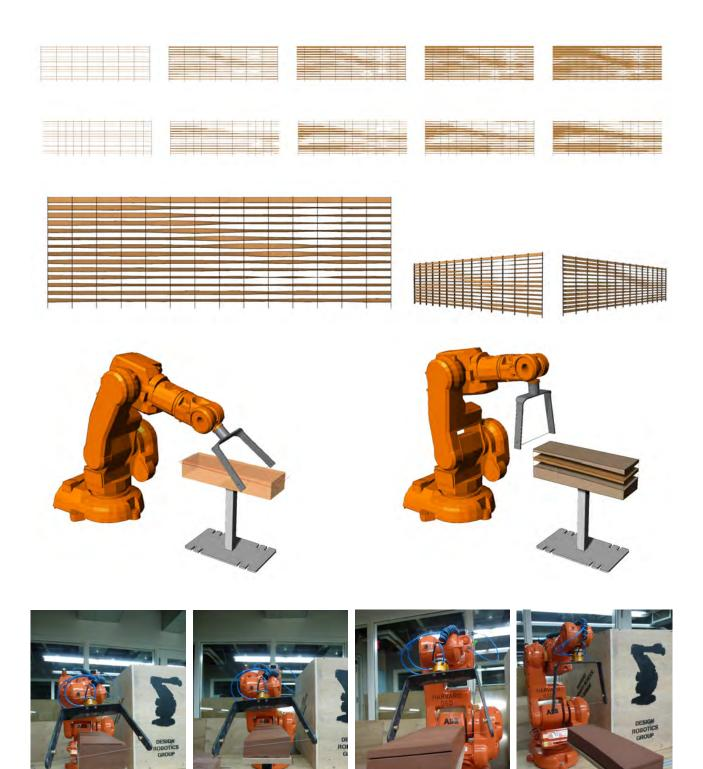
Fig. 8: Pattern design and robotic wire-cutting of curved louvers for kinetic shading systems.
