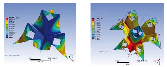
Fig. 6: Deformation patterns after structural analysis exhibit analogous rotational symmetries with the synthesis process.
