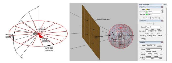
Fig. 4: Instrumental resolution and real resolution
