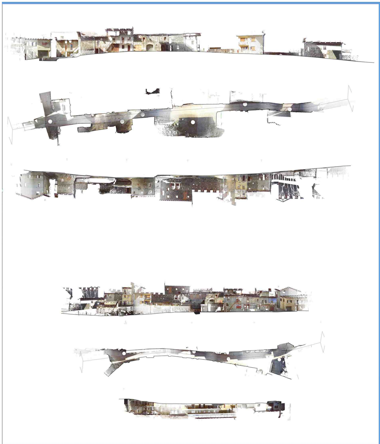
Fig. 5: Survey performed with the laser scanner of the fronts and of the planimetric development of the ricetto 's two streets.
