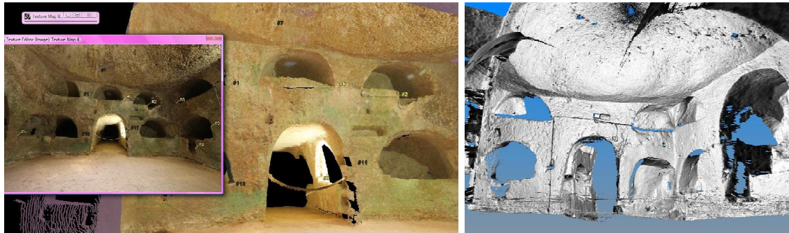
Fig. 11-12: Texture mapping(left) and mesh model (right) of the cubicle of Eusebio
