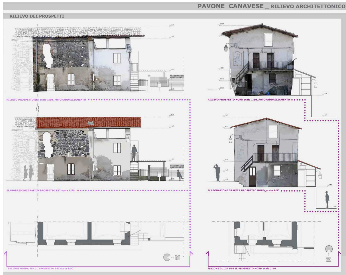
Fig. 6: Survey of one of the buildings of the ricetto , made with the integration of the results obtained through the analytical straightening of digital images and the direct survey. This representation highlights the presence of different textures walls, showing the transformations that have occurred over the centuries.
