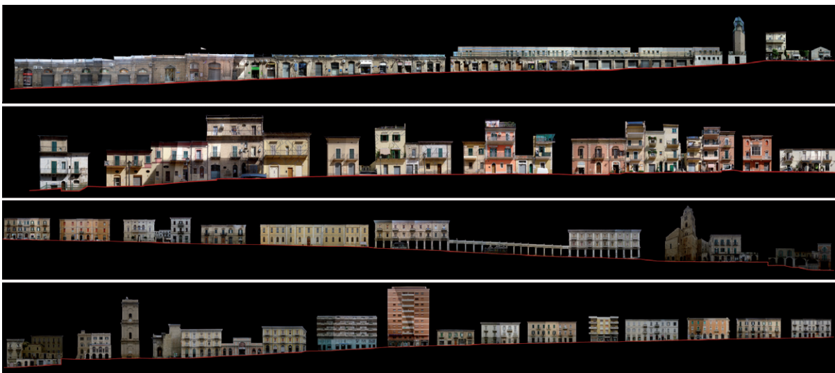
Fig. 6: Surveying the Fiera District. Photo-straightening: via Monte Maiella and corso Trento e Trieste, both sides.
