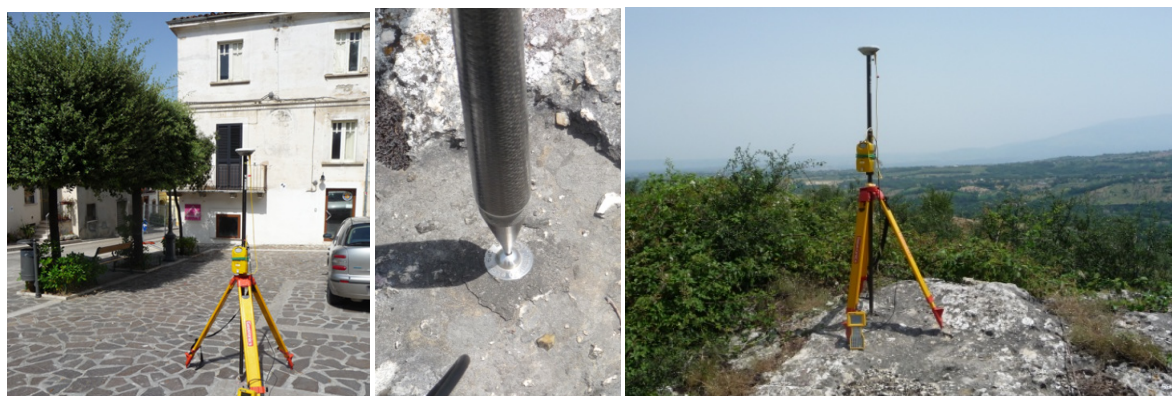
Fig. 2: Topographic surveys, identification and materialization of points with GPS.
