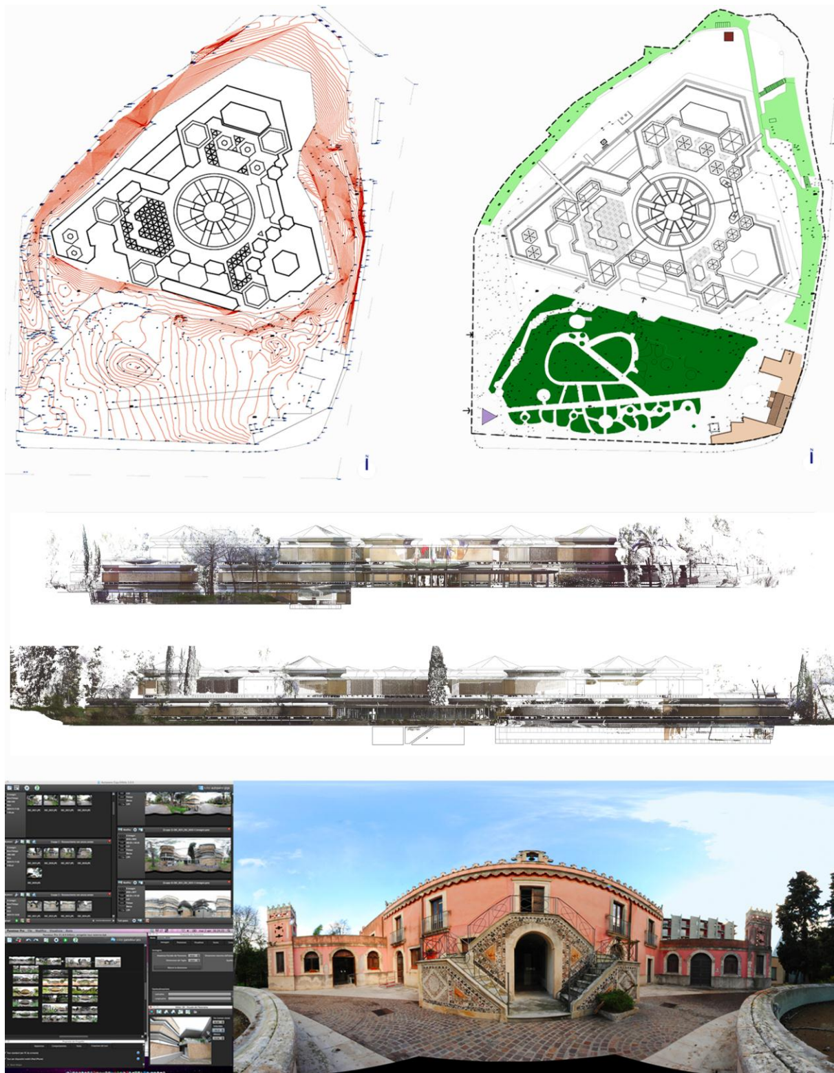
Fig. 3: Images from the integrated survey: urban plan acquired by GPS (a), orthographic projections obtained by 3D laser scanning (b) and panoramic virtual tour realized by photo sticking (c).
