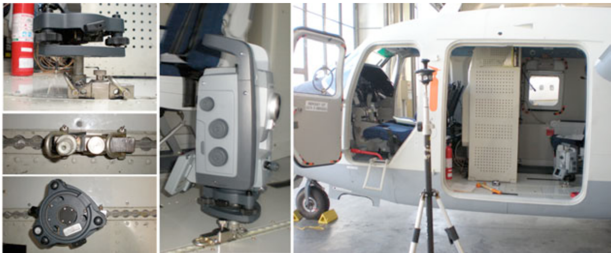
Fig. 5: Topographic survey by Total Station type Trimble VX in order to measure physical offsets between the sensors installed on board the aircraft. Support of the Total Station VX designed by university researchers and built by aeronautical engineers of GdIF.
