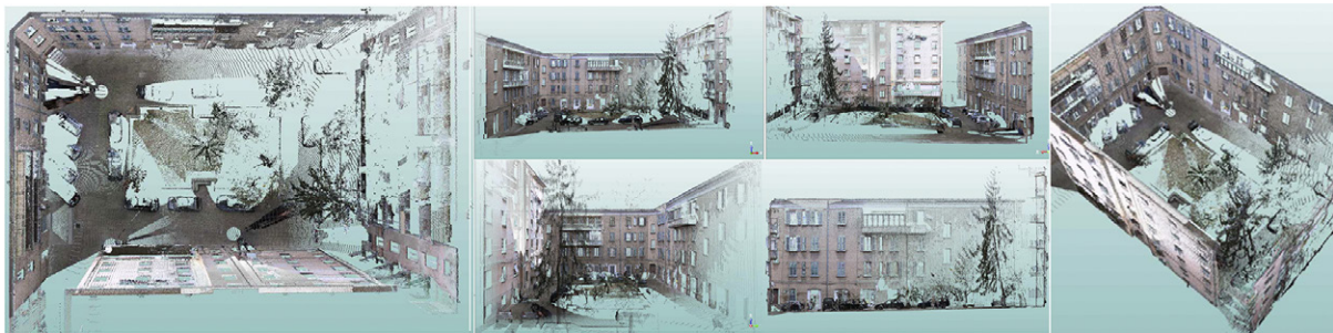
Fig. 5: Surveying the Fiera District. The phases of indirect surveying included a laser scanning campaign using a Photon 120 scanner coupled with a Nikon D300s camera recording on a dedicated hard disk.
