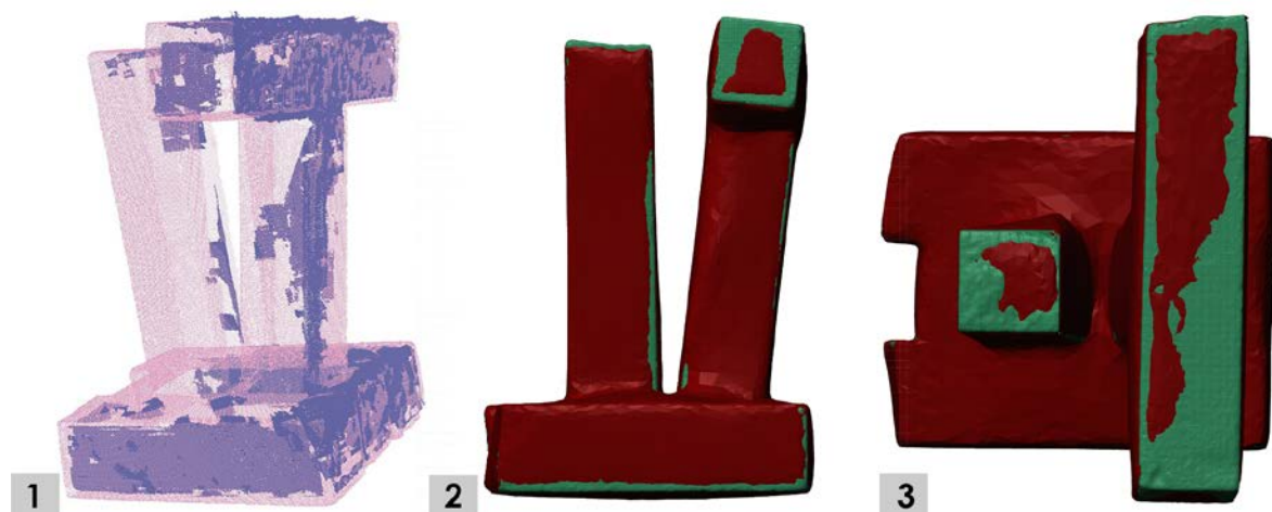
Fig. 7: [1] Overlapping point clouds obtained from Shape from Stereo method (darker) versus Laser Scanner Data (lighter); [2 and 3] Side and top views of the overlapping meshes: Shape from Silhouette mesh in red versus Laser Scanner Data mesh in green.
