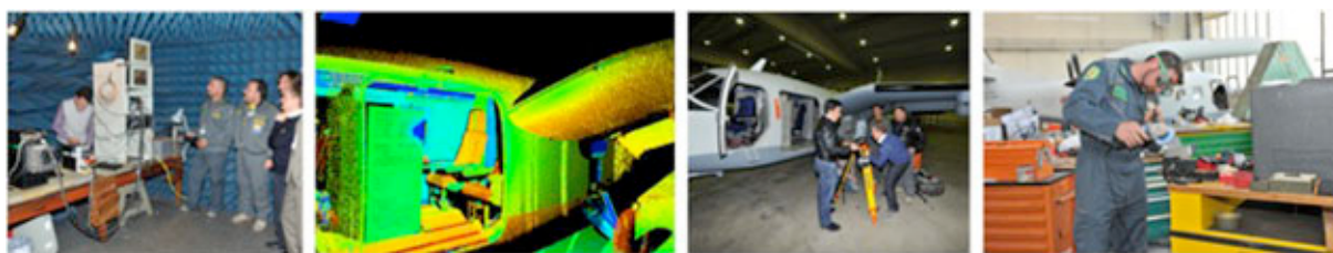
Fig. 2: Four preliminary phases to the first flight of remote sensing: the electromagnetic test in an anechoic room, 3D point cloud model of the aircraft, the sensors calibration, the improvement of the installation components.
