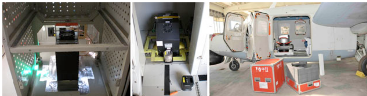
Fig. 2: Airborne digital sensors: from left to right, Itres TABI-320 and CASI-1500, ready for remote sensing missions; Leica ADS40 during installation tests.
