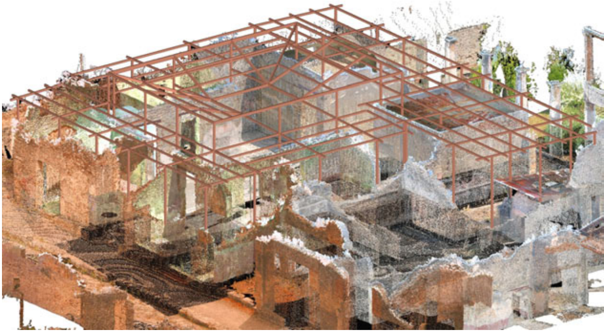
Fig. 7: Model of the load-bearing structure of the hypothetical steel roofing within the point cloud data.
