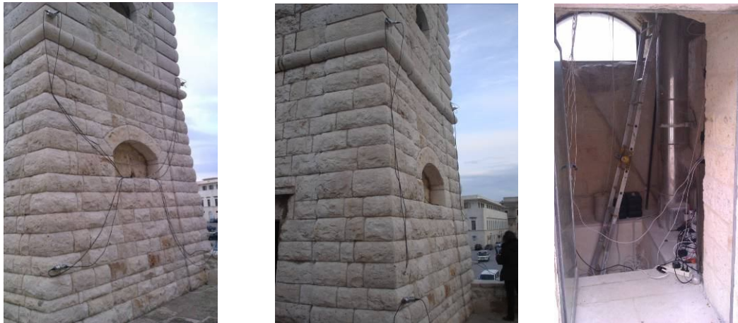
Fig. 2: Details of the accelerometers mounted on the tower and the connecting wires
