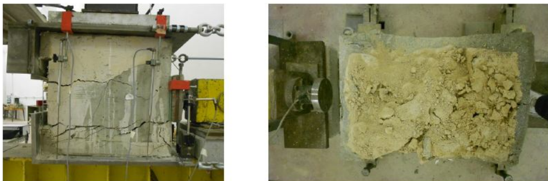
Fig. 12: Typical shear crack pattern on the external reinforcing SCC (left) and view of the specimen after test, with the fiber reinforced SCC plaster not debonded from the internal masonry core (right).
