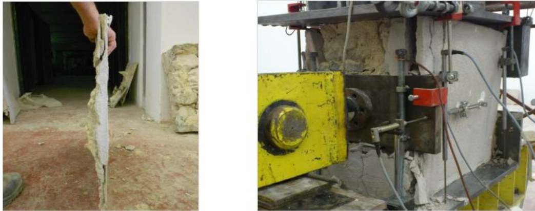
Fig. 11: Detachment of the plaster in wall specimens reinforced with mesh.
