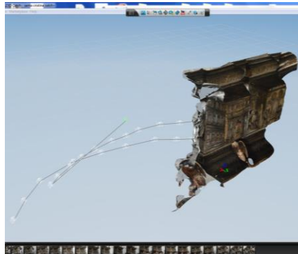
Fig. 2: 123D Catch data set and wireframe visualization of OBJ model of a part of S. Cristina urn in Dome of Palermo
