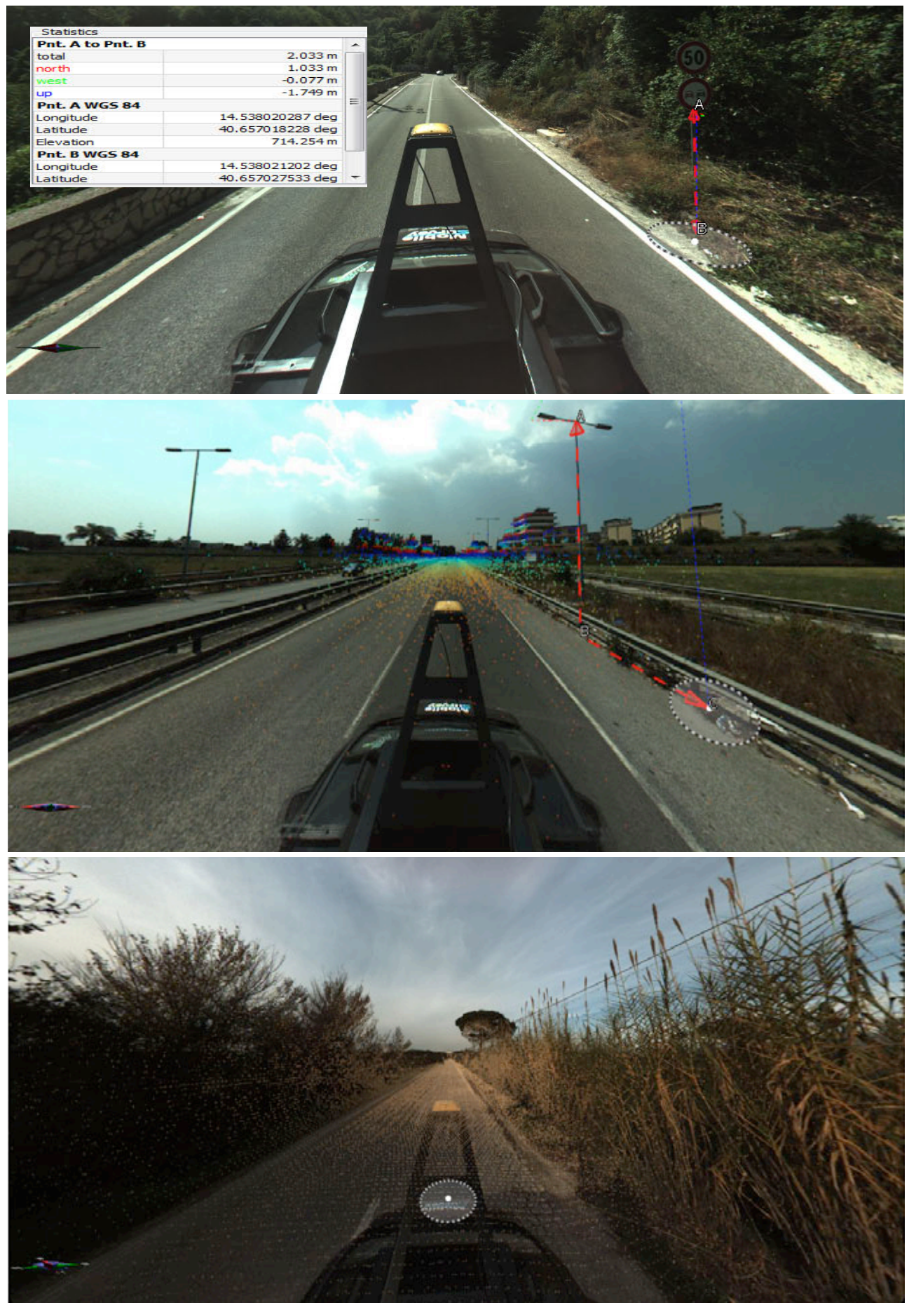
Fig. 2: Extraction of geometric informations about the elements of the road section.
