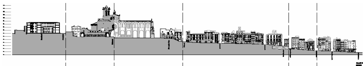
Figure 7: Section of the hill of Tarragona (“Part alta”) through the cloister and the nave of the Cathedral.
