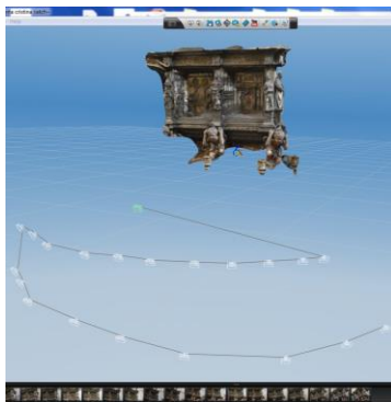
Fig. 2: 123D Catch data set and wireframe visualization of OBJ model of a part of S. Cristina urn in Dome of Palermo
