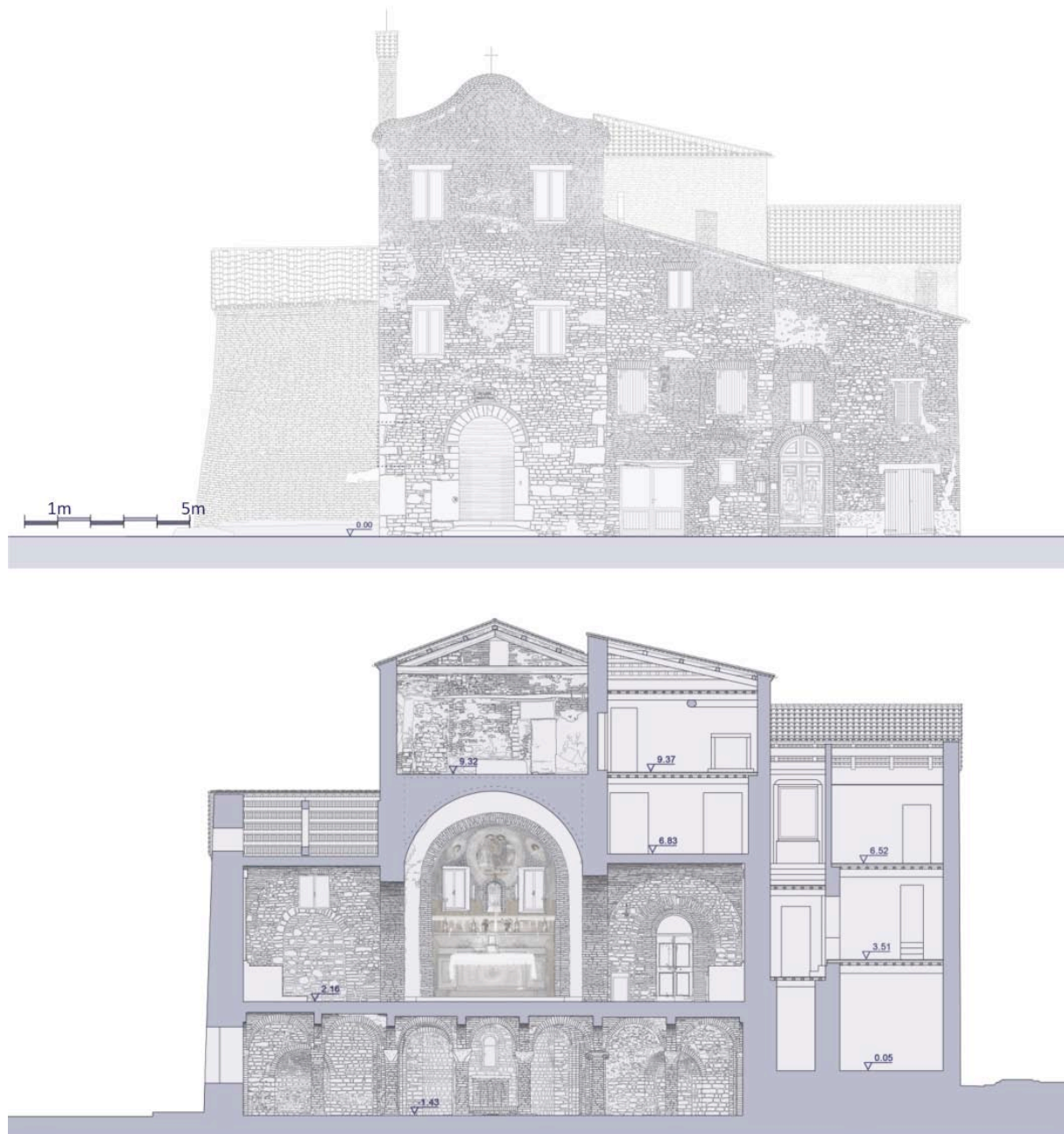
Fig. 7-8: Principal perspective and cross-section; the texture was processed in Autocad after photo-straightening was complete. Such a section of the transept highlights the three-level system: crypt, church, and upper environment.
