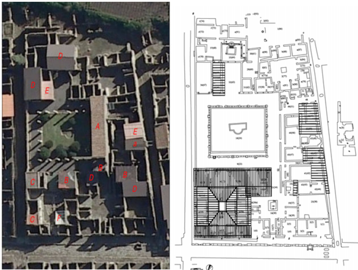
Fig. 1: On the left the existing roof coverings of the Insula of the Centenary (zenithal view from Bing Maps 2010), on the right the design indications for the new, hypothetical roof coverings with a structure made of aluminium and a roof covering made of polycarbonate.
