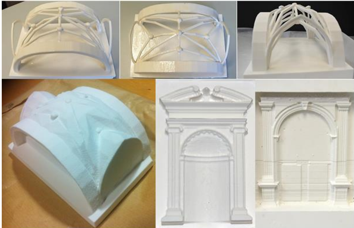
Fig. 11: Views of the physical models made using a 3D printer in the case of the vaults and using of numeric control milling in the case of the front and niches.
