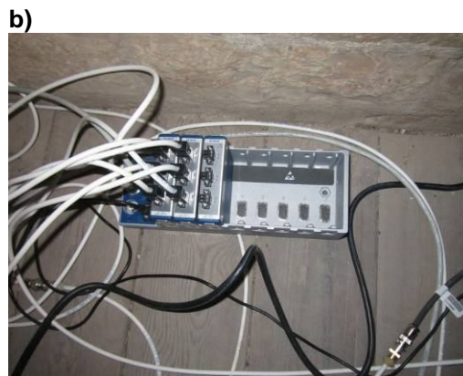
Fig. 5: a) example of piezoelectric accelerometers, PCB National Instruments; b) acquisition modules (DAQ).
