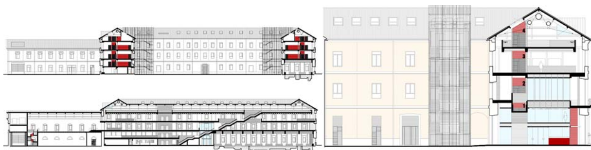
Fig. 5: LRC project. Longitudinal sections by the main space, by the courtyard and transversal section E-W by the main entrance and the courtyard.
