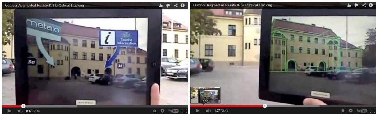
Fig. 3: Metaio experimental markless system based on geometry of the site.
