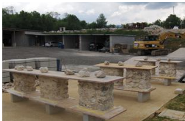
Fig. 6: Reconstructed wall masonry specimens.
