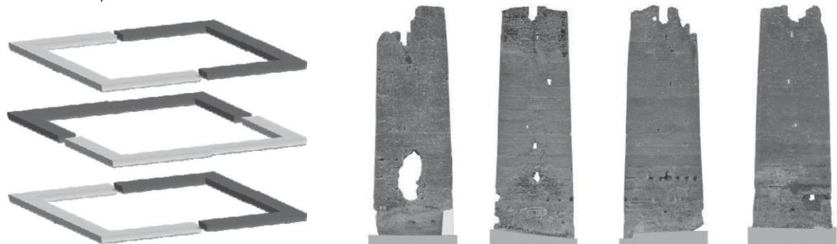
Fig. 10: Building system used alternating the available "U" shaped formwork (Vegas & Mileto)
