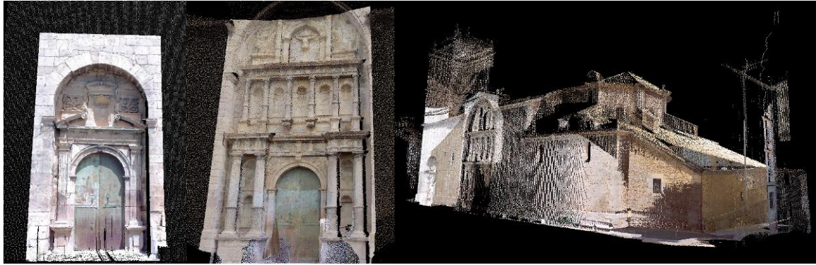
Fig. 5: Views of the assembly point cloud from scans with different densities of the principal facades and their covers.
