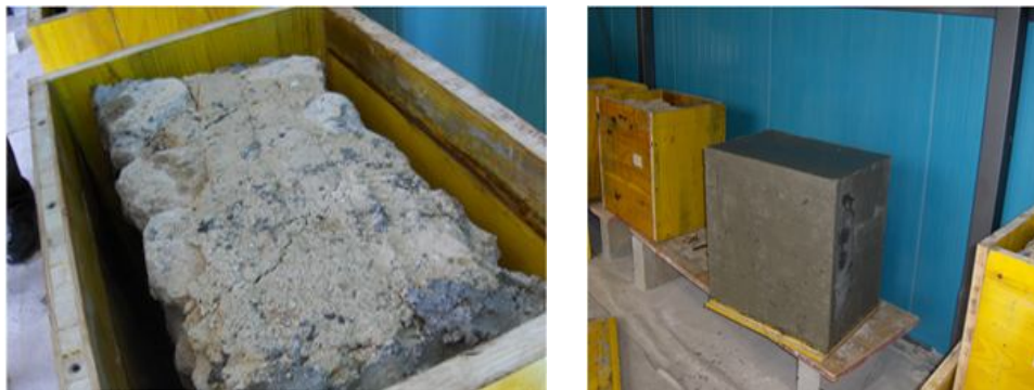
Fig. 7: Wall specimen: before casting of the reinforced plaster (left) and after curing (right).
