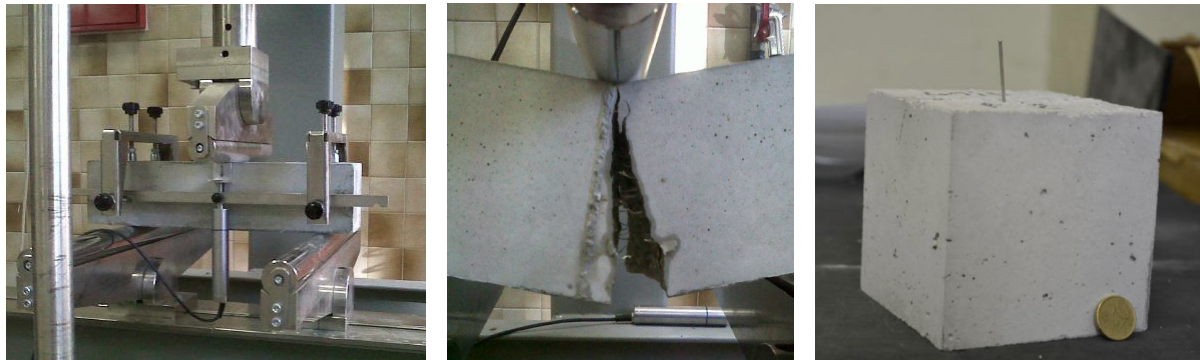
Fig. 4: Three point bending test (left and middle), fiber in concrete cube for pull-out test of a single fiber (right).
