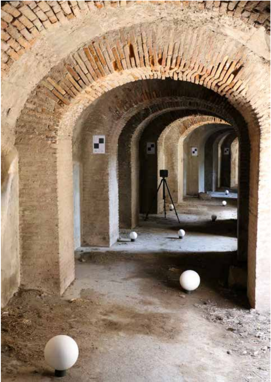
Pompeii, Amphitheater. 3D Laser Scanner capturing in the underground tunnel.
