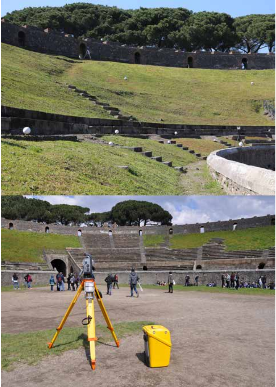
Pompeii, Amphitheater. 3D Laser Scanners capturing, and topographical acquisition.
