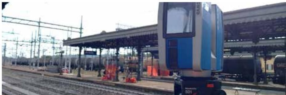
6 Scansioni banchina con Laser Scanner Faro Focus 3D X330 HDR
